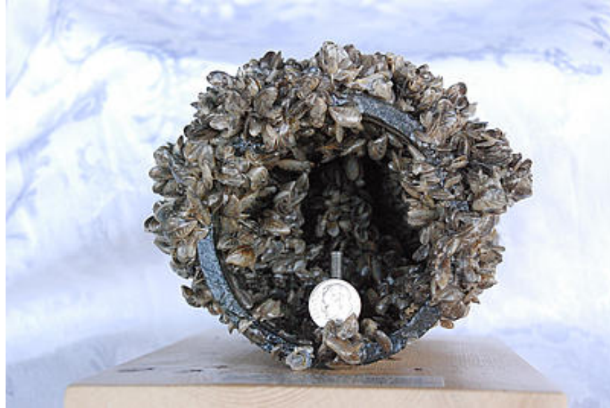
Figure 2. Photograph of quagga mussels clogging a pipe. Note the dime in the foreground of the photo for scale. Photo found at http://www.pe.com/imagesdaily/2009/05-21/quagga21_400.jpg (June 2011).
