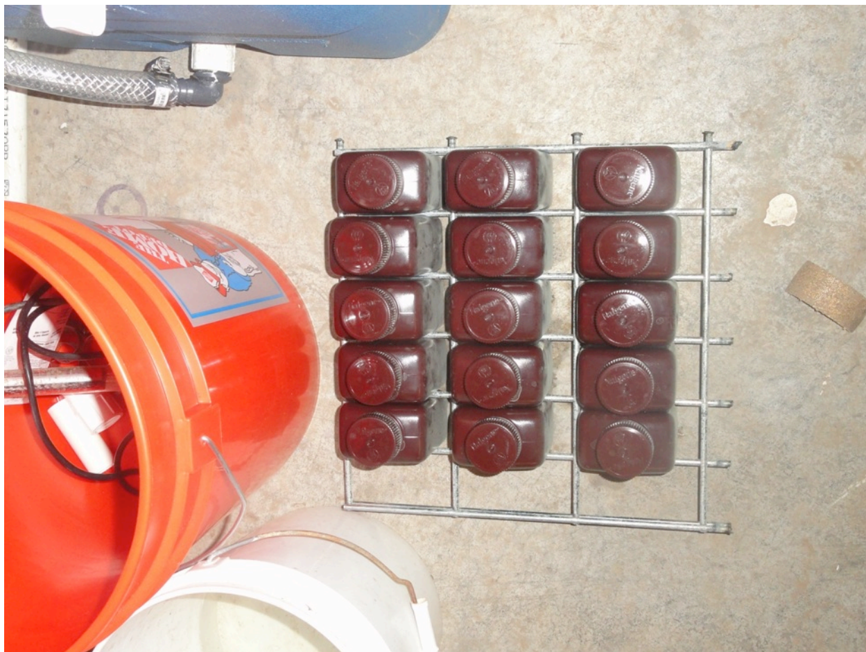
Figure 5. Photograph of the screen apparatus used to hold bottles within each cooler.
