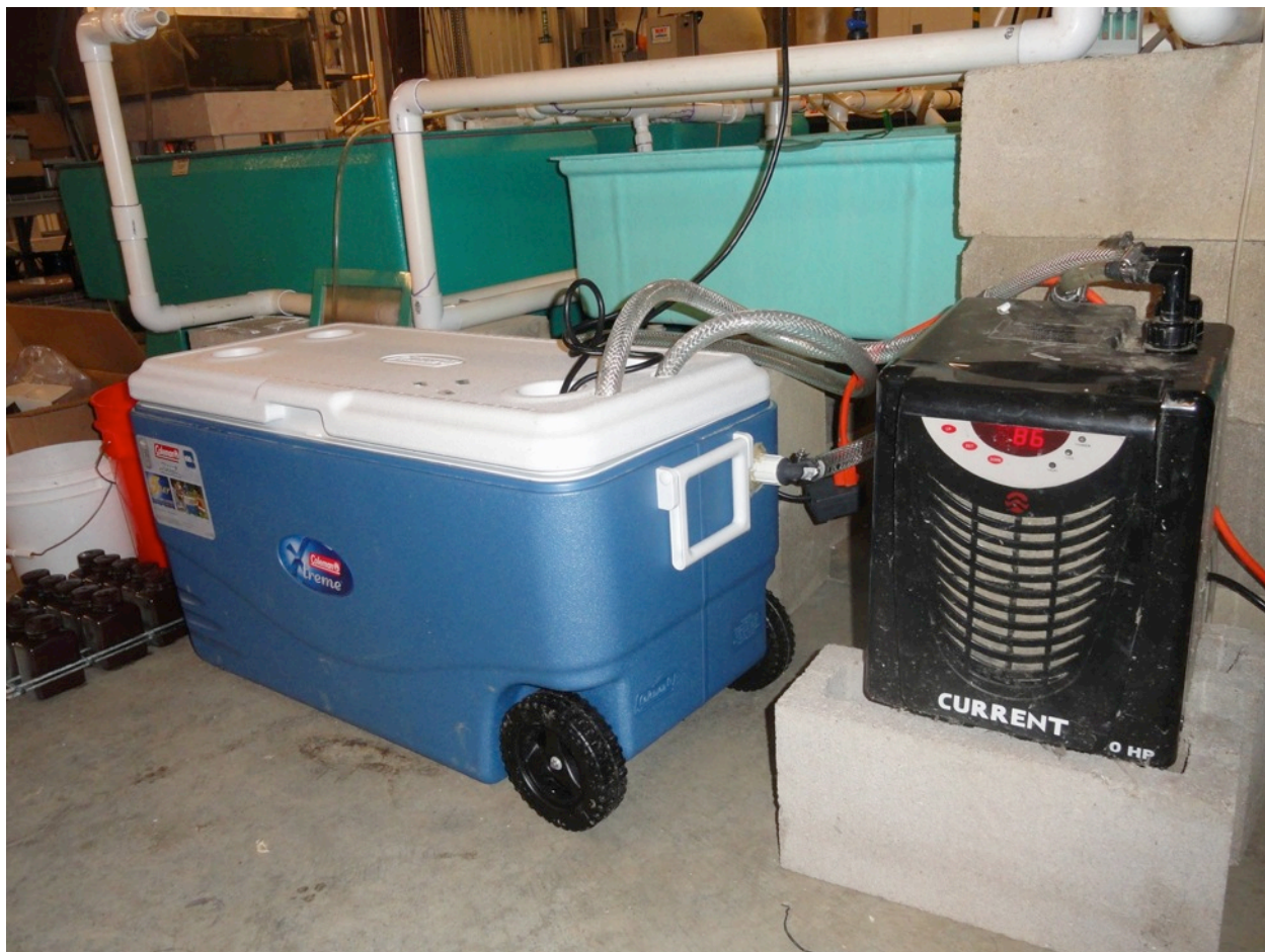
Figure 3. Photograph of the cooler, chiller, and heater system used for each temperature treatment.
