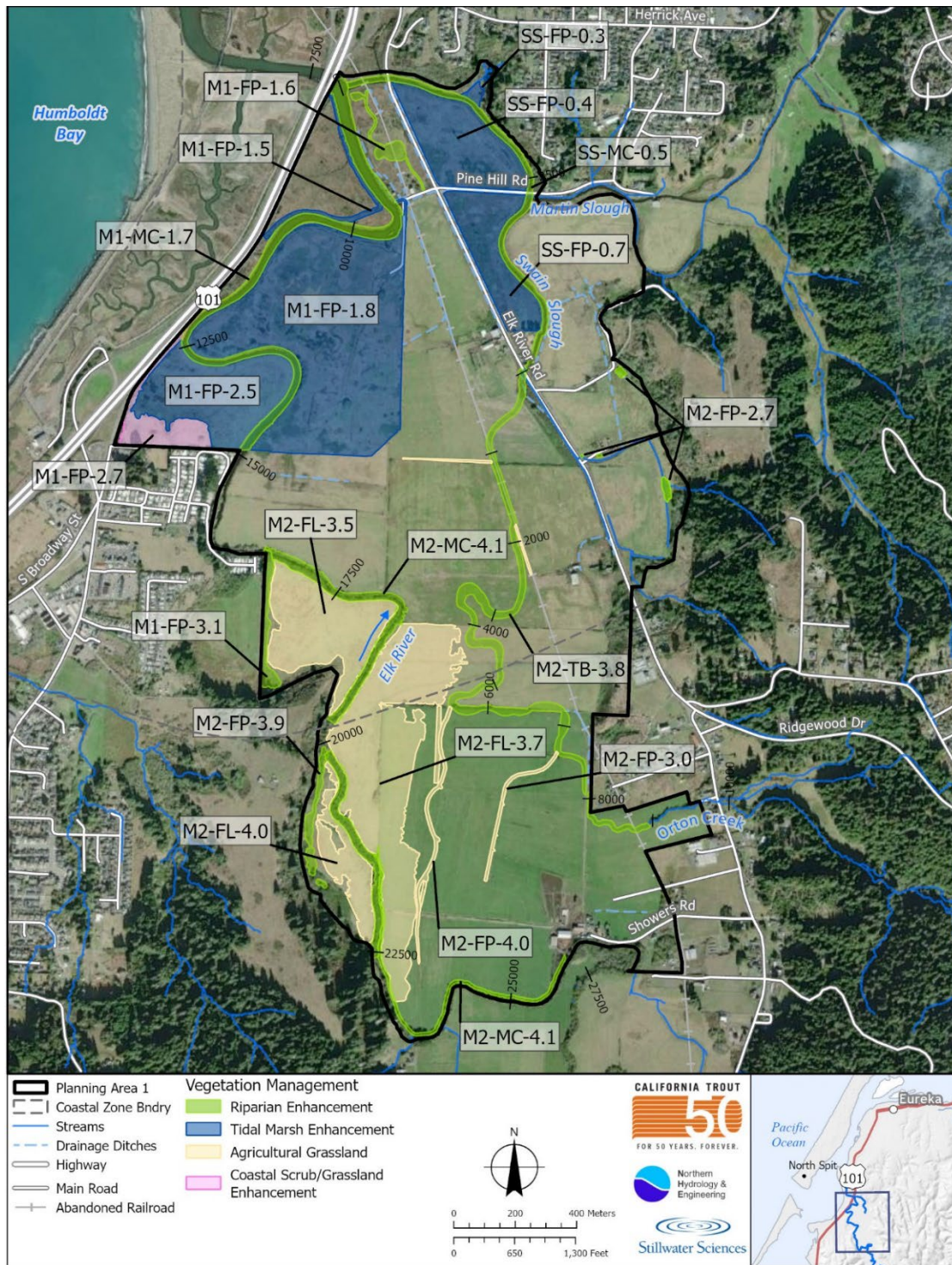
Figure 3-17. Vegetation actions in the enhancement sites include post-disturbance revegetation of sediment reuse areas to re-establish grasslands for grazing and excavated floodplain swales, conversion of agricultural grasslands to riparian forests along mainstem Elk River and the new alignment of Orton Creek, thinning and interplanting of vegetation along mainstem Elk River to improve diversity and wildlife habitat, and conversion of agricultural grasslands to tidal marsh at tidal marsh enhancement sites.
