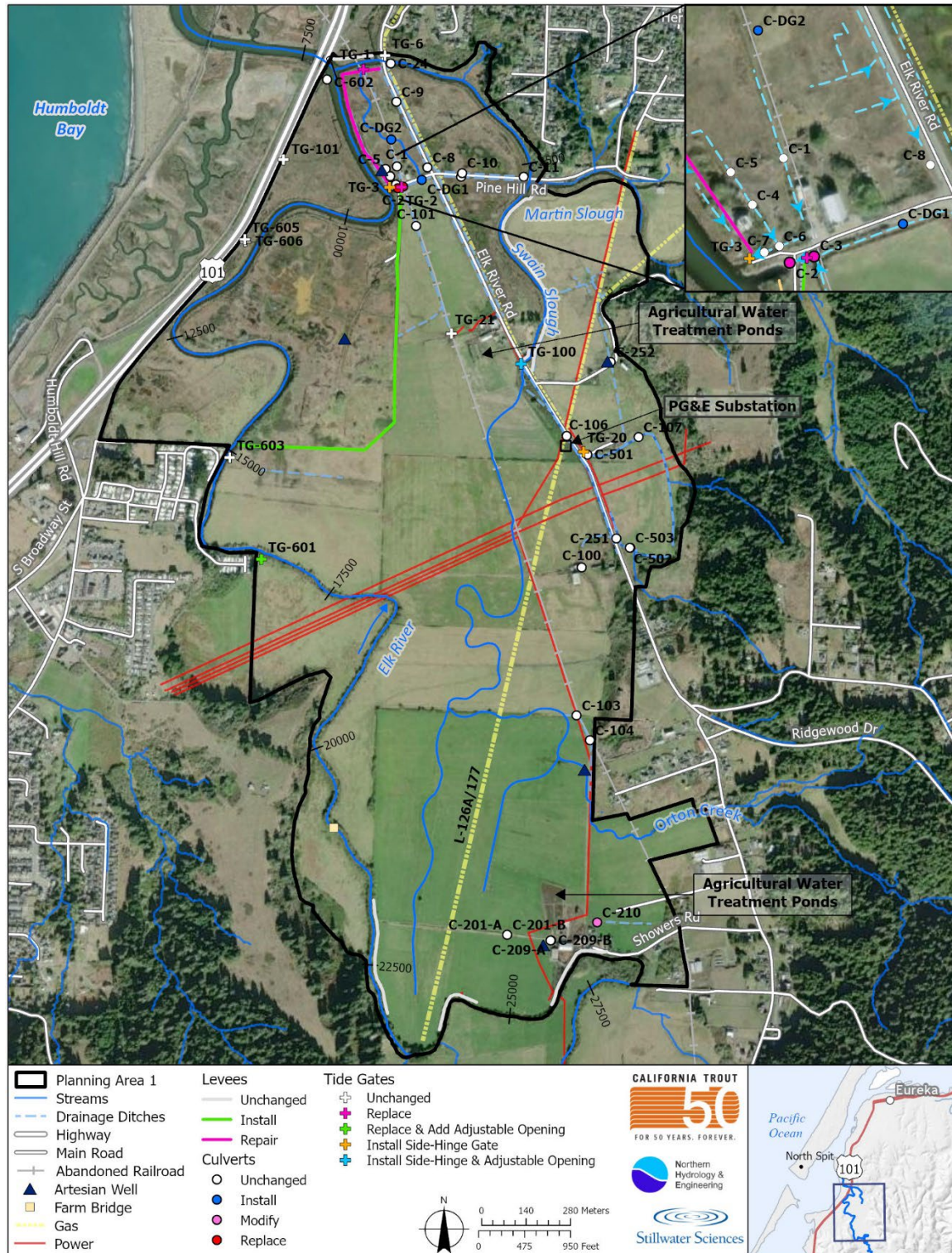
Figure 3-16. Proposed new infrastructure includes installing larger tide gates (side-hinge with optional ability to allow a muted tide at select sites), culvert through Pine Hill Road to improve drainage, increase existing levee height to protect freshwater off-channel enhancement site, eco-berm to protect agricultural lands while allowing full tidal restoration.
