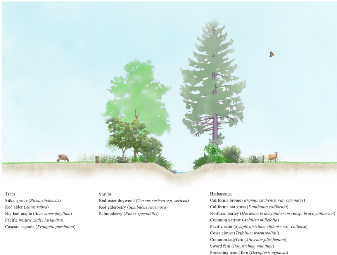
Figure 3-13. Tributary restoration may include daylighting tributaries that flow through long culverts, riparian enhancement, improving channel complexity wood, alcoves, inset benches, and exclusion fencing. Some riparian areas may be suitable for flash grazing as shown. Example is from Orton Creek in PA1.
