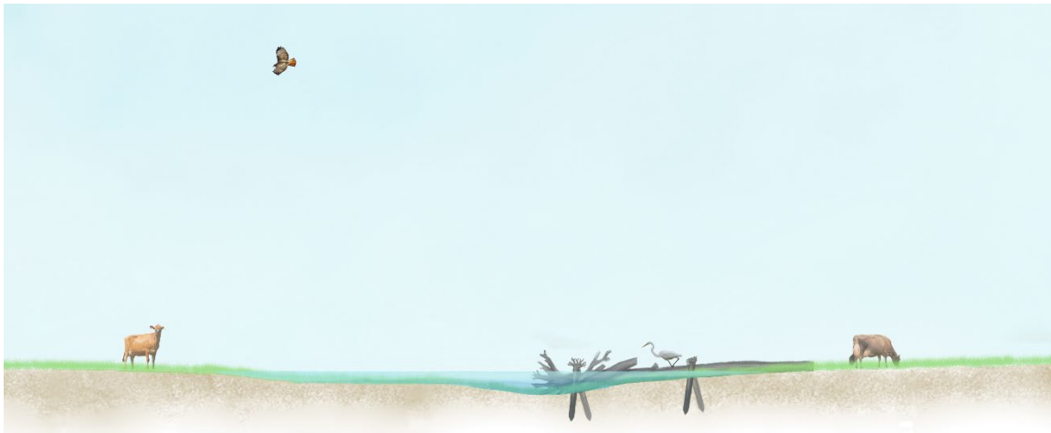
Figure 3-12. Floodplain channel through agricultural grasslands during flood flows in the Elk River. The low flow channel, set within a broad shallow floodplain channel, provides deeper flow paths with cover for fish to pass through agricultural grasslands to reach higher quality habitats as high water recedes. During dry periods, the floodplain channel is grazed.
