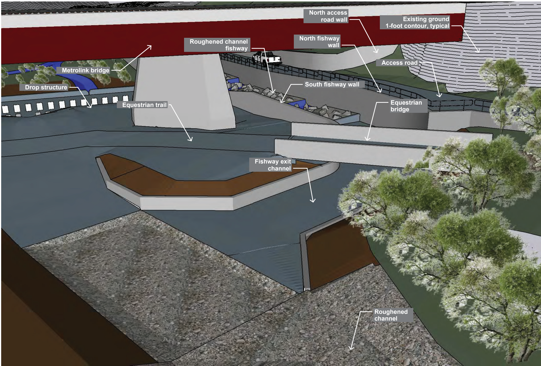
Perspective view of 3D rendering fishway exit channel and drop structure split, looking downstream
