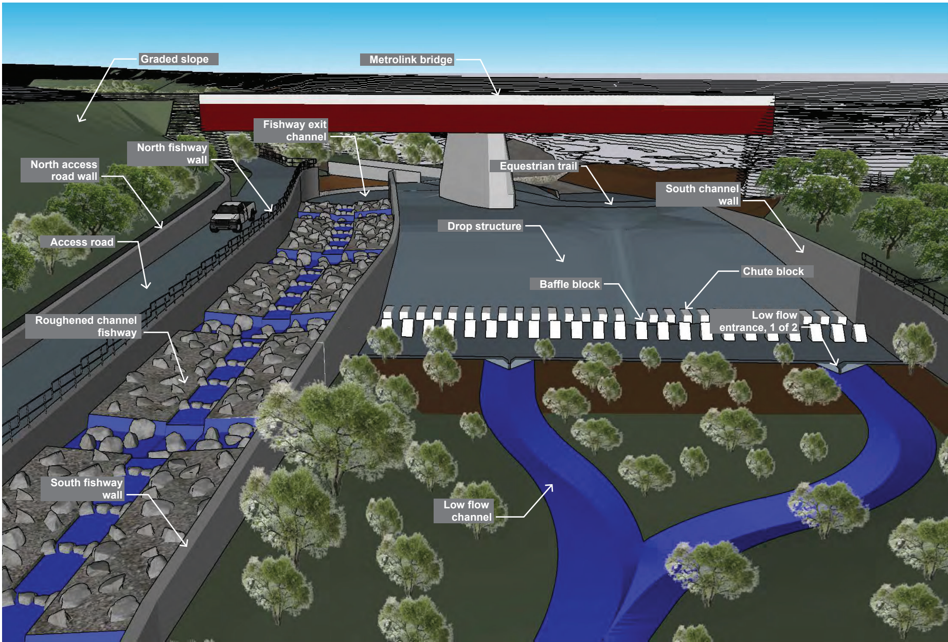
Perspective view of 3D rendering showing the proposed project, looking upstream from midway down the fishway
